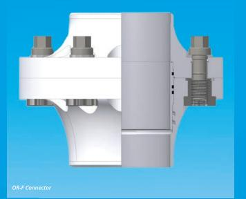
OR-F flanged risers are supplied in lengths from 5 ft. pup joint to full length 90 ft. joints and can either be slick or fitted with buoyancy. OR-F flanged riser connectors are simple to operate by applying the recommended torque to six main bolts to achieve the required pre-loading.
