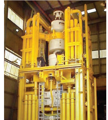
BOP Stack with Subsea Flexible Joint
